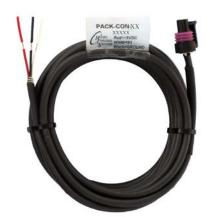
The cable is available in either 20', 40 or 60' lengths with a removable Packard connector to provide easy serviceability. The wire is sealed and crimped to the Packard connector providing a liquid tight environment and strain relief. Media compatibility: Refrigerants (freons) and ammonia.
